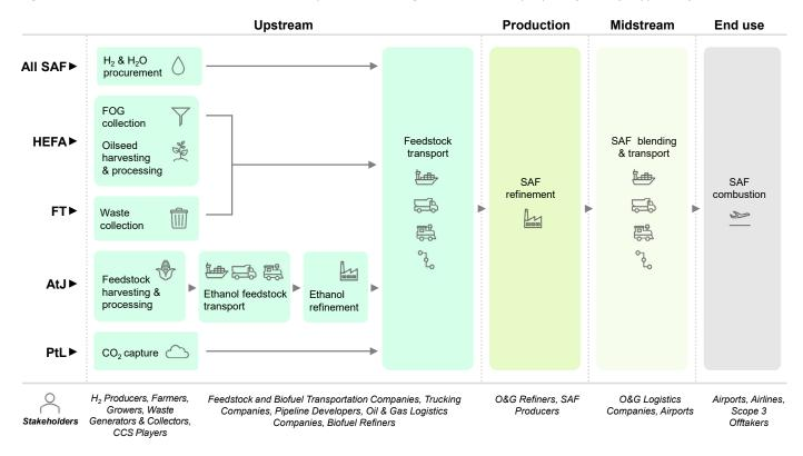
**Hydroprocessed Esters and Fatty Acids (HEFA)** requires triglyceride feedstocks such as oilseeds and waste fats, oils, and greases (FOGs). HEFA is the most mature technology pathway to produce SAF and is the only pathway that has been deployed at commercial scale.
