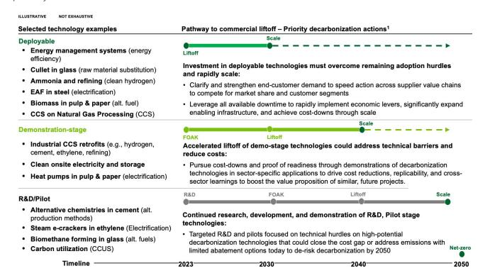
Figure 3a.iii.7: The U.S. industrials pathway to commercial liftoff consists of a series of industry actions across deployable, demonstration-stage, and R&D / pilot-stage technologies. | 1. Indicative timeline presented for R&D, FOAK, liftoff, and scale. Actual timelines will vary by technology based on technological maturity and barriers to adoption.
