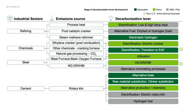
Figure 3a.ii.4: The left and middle columns outline the sources of emissions abated via CCS in this report's MACC results. The right column identifies potential alternative technologies to CCS and their associated stages of deployment.
