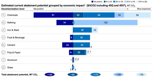
Note: Unabated emissions (~40 MT CO<sub>2</sub>), external factors<sup>5</sup> (~200 MT CO<sub>2</sub>), and abatement potential with costs \$250+ /tCO<sub>2</sub> (~5 MT CO<sub>2</sub>) are not shown in this figure
