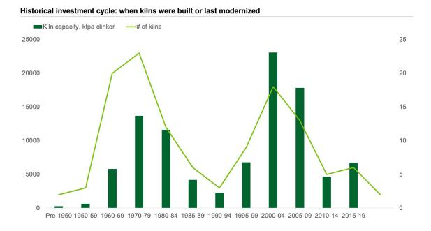
Figure 2.3. Historical investment cycle for cement plants. Number of kilns and capacity by period of construction or most recent modernization. The most recent surge in investment came in 2000–09 when 31 kilns representing ~41 MTPA of clinker-production capacity were built or modernized. Source: Portland Cement Association (2019, Dec. 31). U.S. Portland Cement Industry: Plant Information Summary.
