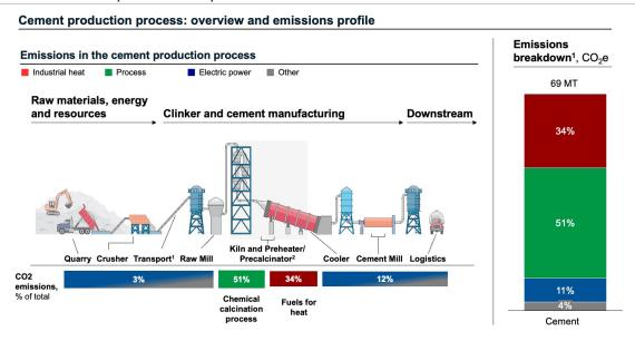
Figure 2.1. Overview of the cement production process with corresponding emissions by source. 85% of emissions come from clinker production in the preheater/precalciner and kiln, of which 51% are intrinsic to the chemical calcination process and 34% come from the combustion of fuels for heat.
